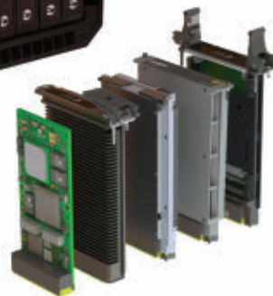
Agnostic OpenVPX embedded computing cooling technology from Mercury Systems can be packaged as circuit board-only, Air Flow-By and Liquid Flow-By, conduction cooled and Liquid Flow-Through, Air Flow-Through, and convection cooled.
