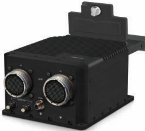
General Micro Systems uses a proprietary thermal-management technology called RuggedCool for HPEC applications to cool 300-Watt Intel Xeon processors.
